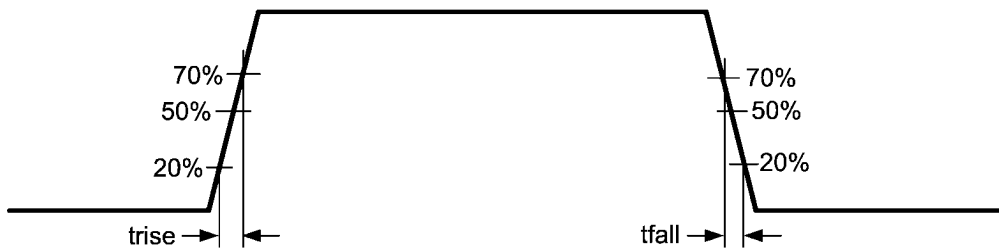
FIGURE 2. Output Transition Time (A and B Side)
